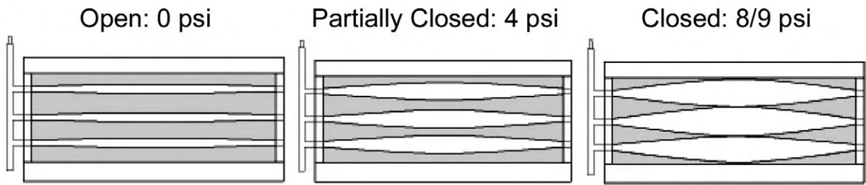
Figure 8.17: Pneumatic (“Bladder”) Damper
