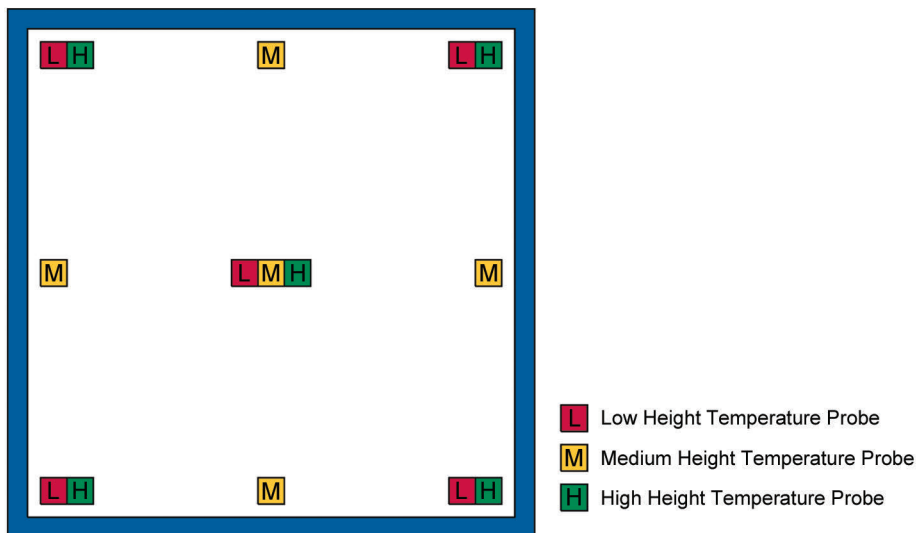
Figure 18.2: Mapping Locations for a CRT Space up to 700 cubic feet (20 cubic meters)
