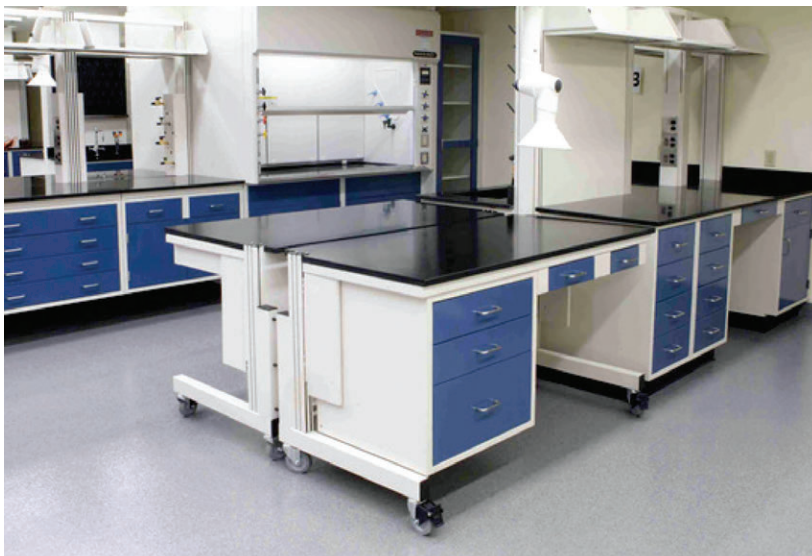
Figure 7.5b: C-Frame Casework Designed to Move About Lab; Suspended Casework in Background
