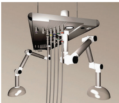
Figure 7.7: Schematic of Overhead Service Carrier
