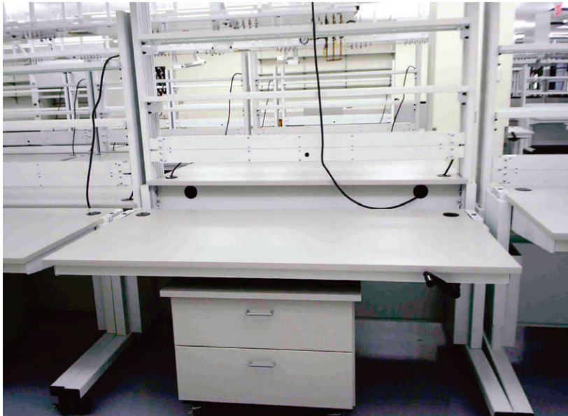
Figure 7.5a: C-Frame Casework with Movable Storage Under
